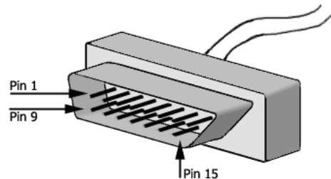
Servo Animator does not currently support the joystick buttons or Joystick 2 Y. To assemble your input device, connect a 100K Ohm variable resistor between +5V and the input pin that you are using. (ex: Joystick 1 X) Use any sort of mechanical apparatus to move your variable resistor and you will be able to use that to animate.
